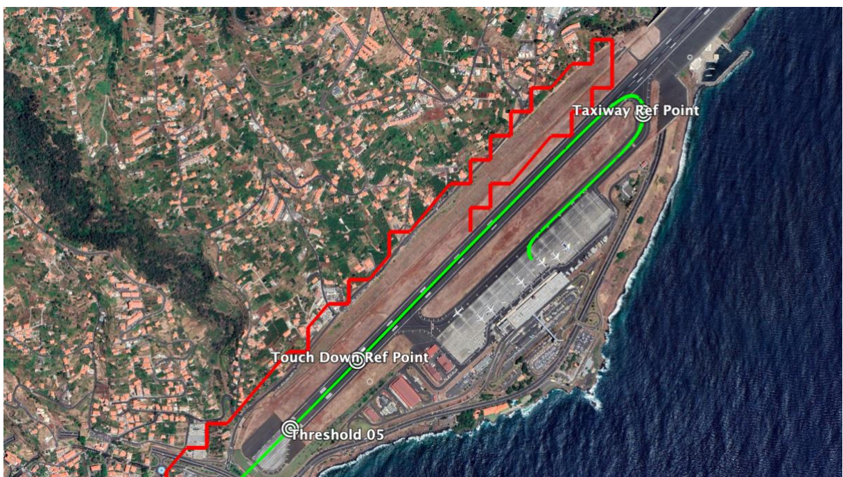
Figure 3.5 – In green an example of the horizontal projection of the flight path after RTS smoothing and adjustment. The points referenced are used for Local Coordinate System origin (Threshold 05) and trajectory shifting (Touchdown and Taxiway)[Image source: Google Earth®].
